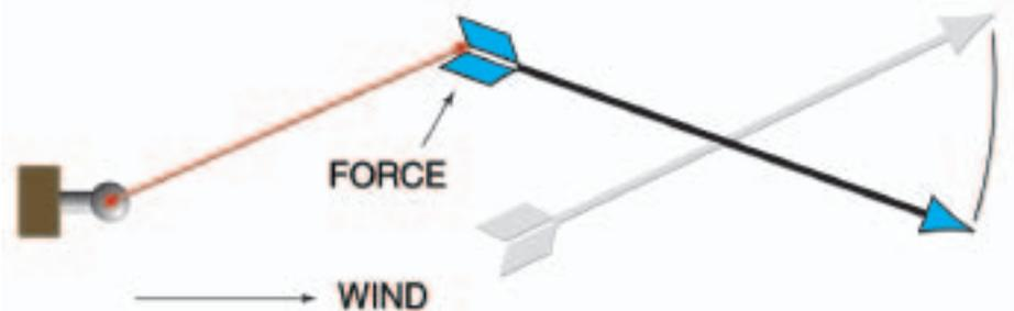
The motion of an arrow is influenced only by air forces. However, the motion of a sailing yacht is influenced by both air and water forces. All sailing yachts are designed to be stable when moving forward through the water. Therefore, they automatically will be unstable when moving astern through the water, as any skipper who attempts to steer the boat backward will attest. The boat will yaw.
